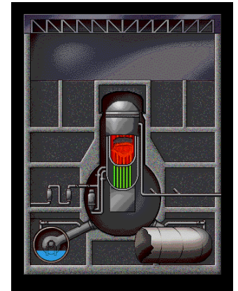
Core Damaged but retained in vessel
