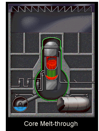
Some portions of core melt into lower RPV
