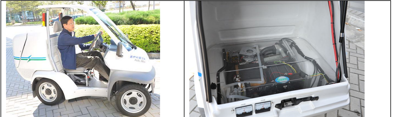
Images: a) delivery 'buggy' developed by APFCT with canisters below driver's seat & b) close-up of the fuel cell stack in the boot.
