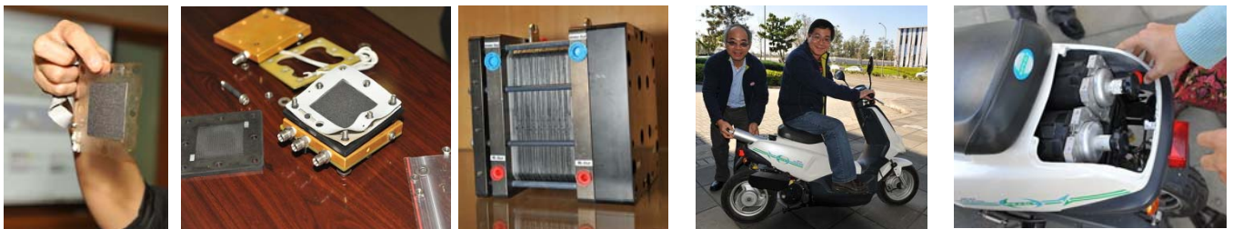
Images: a) APFCT PEM Nafion membrane -Du Pont b) + c) APFCT stacks d) the APFCT scooter & e) rear dual canister hydrogen store
