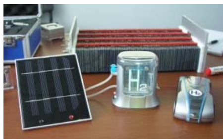
PV to produce electricity for the electrolysis of water to produce hydrogen
